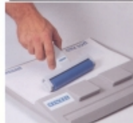
DCR roller being refreshed.
